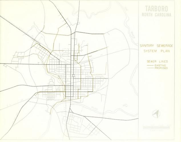
result, considerable infiltration and leakage of storm water into the system has occurred. New lines are presently being installed and connected to the existing pipes. These newly built lines will extend to and replace the three existing lift stations.
